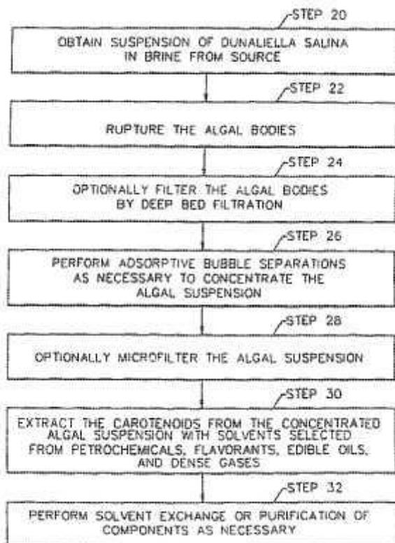
A process and system are disclosed for recovering mixed carotenoids from the alga Dunaliella salina. The harvested cells are ruptured, typically by circulating the algal
